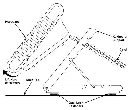
To remove the keyboard from the stand, lift the keyboard from the bottom.
